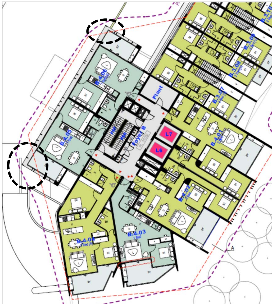
Figure 21: Balcony elements on Building B outside of the approved envelope
